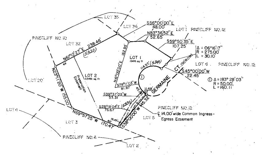
EASEMENTS: Unless shown greater in width, both sides of all side lot lines are hereby platted with a five (5) foot easement for public utilities only, and both sides of all rear lot lines are hereby platted with a seven (7) foot easement for drainage purposes and public utilities only, with the sole responsibility for maintenance being vested with adjacent property owners.
